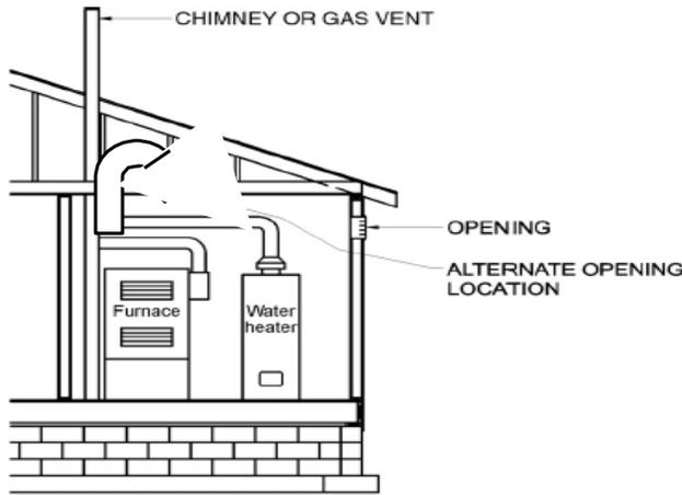
Figure G2407.6.2 is hereby amended to bypass the attic with a duct directly to the outdoors (through the attic).
