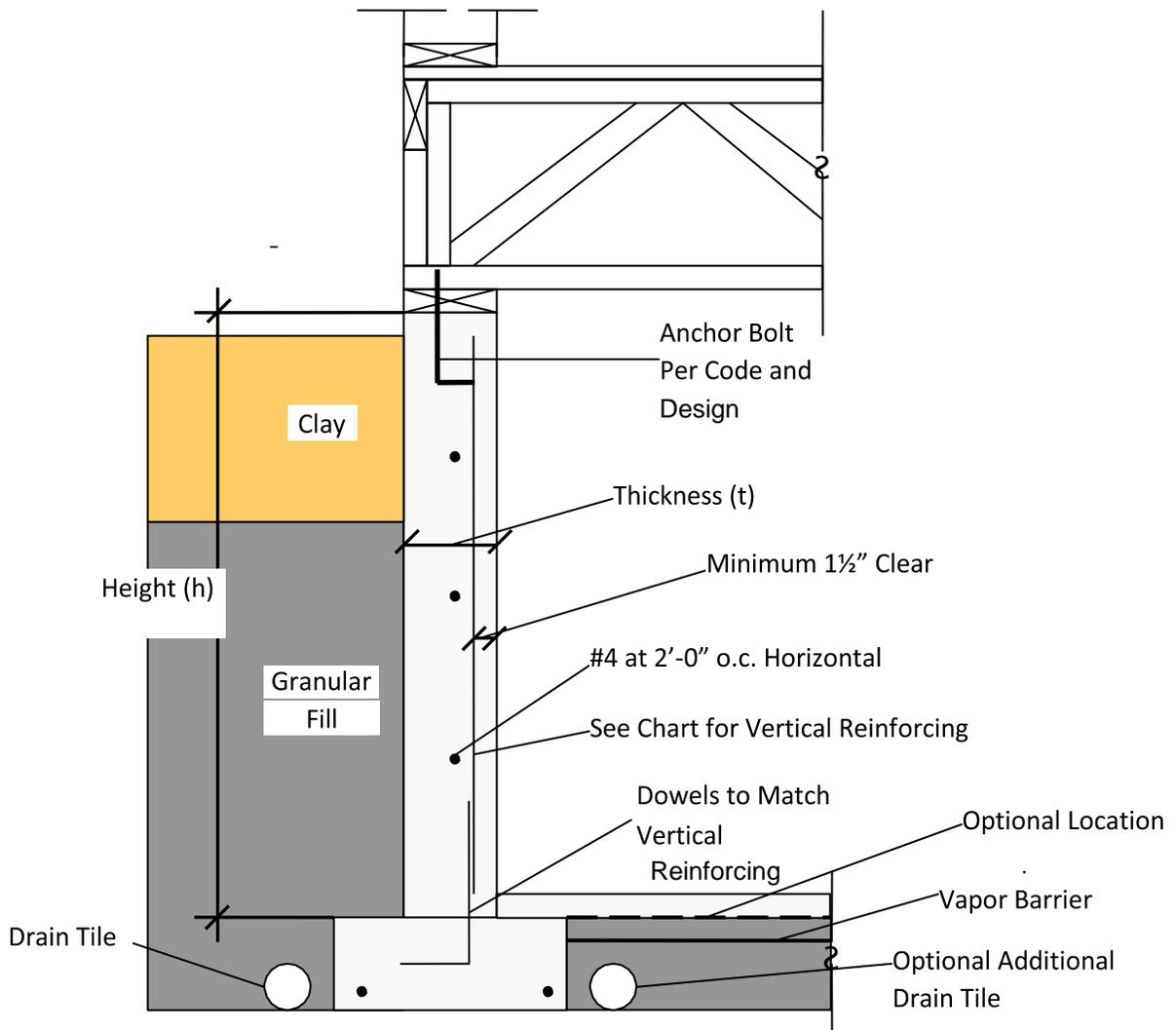
**FIGURE R404.1.2(2), referred to in Section 404.1.2**
